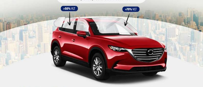
For Wind Screen & Rear Glasses: Provide not less than 70% VLT( Visible Light Transmission )
